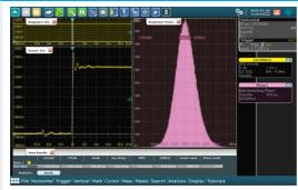
R&S\*RTO oscilloscopes offer over 90 measurement functions. The functions are organized by type into amplitude and time measurements, jitter, eye, histogram and spectral measurements. Statistics, histograms, and trend and track functions facilitate detailed analysis of the measurement results. The measurement results can also be used in math functions.
