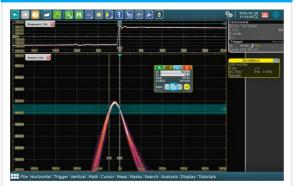
The unique digital trigger system from Rohde & Schwarz minimizes trigger jitter without postprocessing correction. Combined with a high sensitivity that can be extended up to 16 bit in HD mode, you can now reliably isolate even the smallest signals.
