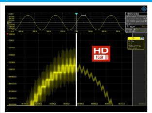
The high definition mode (HD mode) increases the vertical resolution of the R&S\*RTO2000 to up to 16 bit. This results in sharper waveforms, showing signal details that would otherwise be masked by noise.
