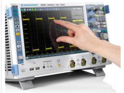
High-resolution capacitive touchscreen allows users to perform functions through gestures.
