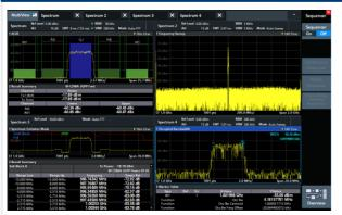
Configure your result windows the way you want. Display multiple measurement channels at once. Sequential channel updating allows e.g. parallel measurement of the spectrum, spectrogram and analog demodulation together with I/Q analysis.
