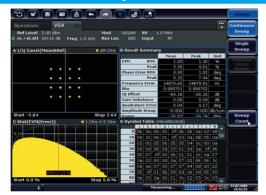
The R&S<sup>®</sup>FPS-K70 option enables users to flexibly configure the analysis of digitally modulated single carriers down to the bit level. The clearly structured operating concept simplifies measurements despite the wide range of analysis tools.
