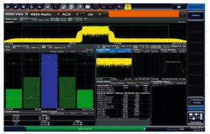
The MSRA simultaneously measures signals of different standards (GSM, WCDMA, LTE, etc.) at different frequencies within its 160 MHz analysis bandwidth.
