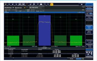
It only takes 1.1 ms to measure the adjacent channel leakage ratio (ACLR) of a 3GPP WCDMA signal.
